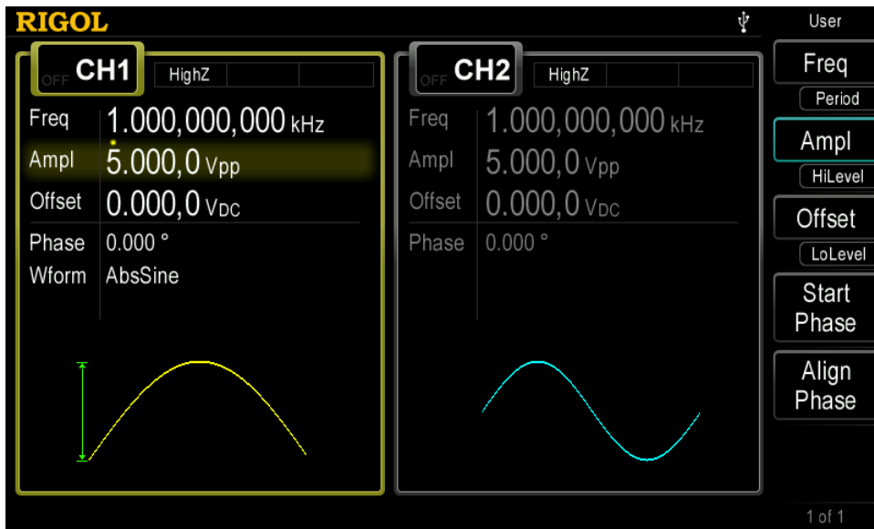
Figure 10-7 Press User Key to Quickly Edit Waveform Parameters
